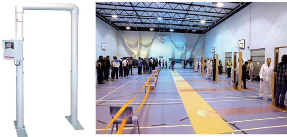
Figure 5: Portal monitor [Canberra Inc. (Left) and IAEA (Right)]
