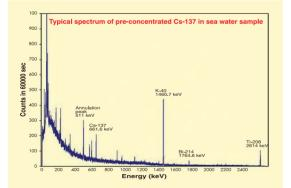
Figure 3. Typical Spectrum of Pre-concentrated Cs-137 in Seawater Sample
