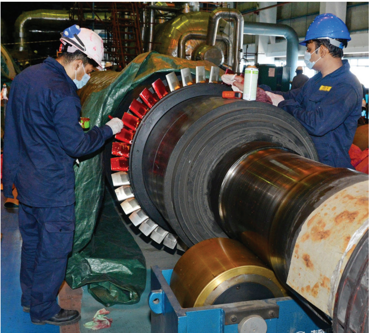
Penetrant testing of generator rotor blades at power plant Source: National Centre for Non-Destructive Testing
