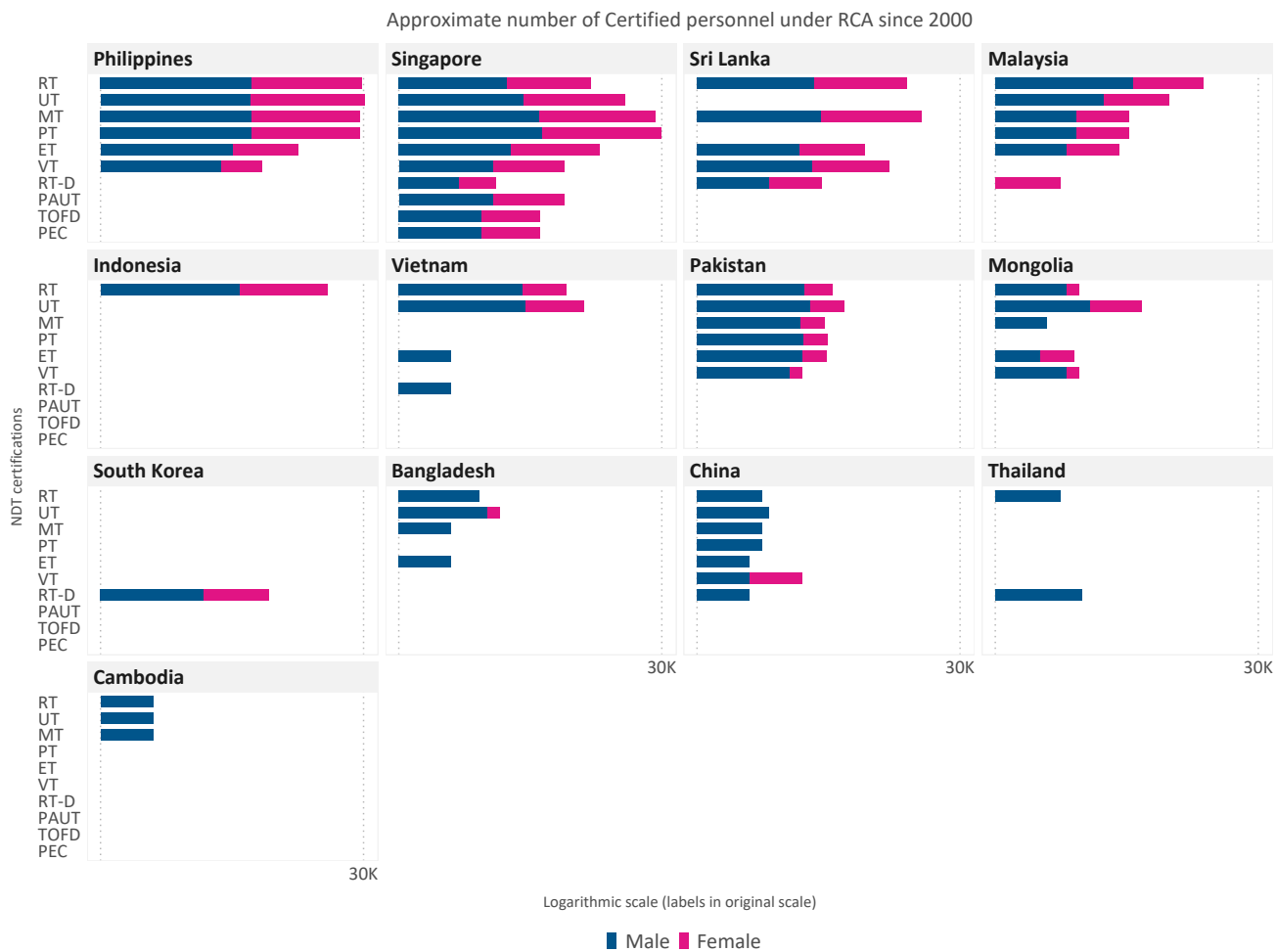
Figure 10: Number of personnel certified by local NDT training centres as a result of participating in the RCA NDT programme
