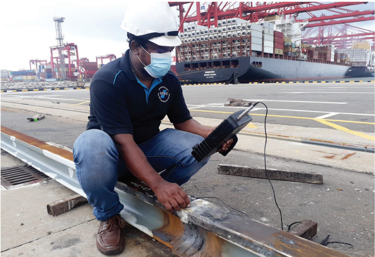
Ultrasonic Testing Inspection on Grantry Rails of East Container Terminals, Sri Lanka Ports Authority, by NCNDT Inspection Team in September 2020. Source: National Centre for Non-Destructive Testing
