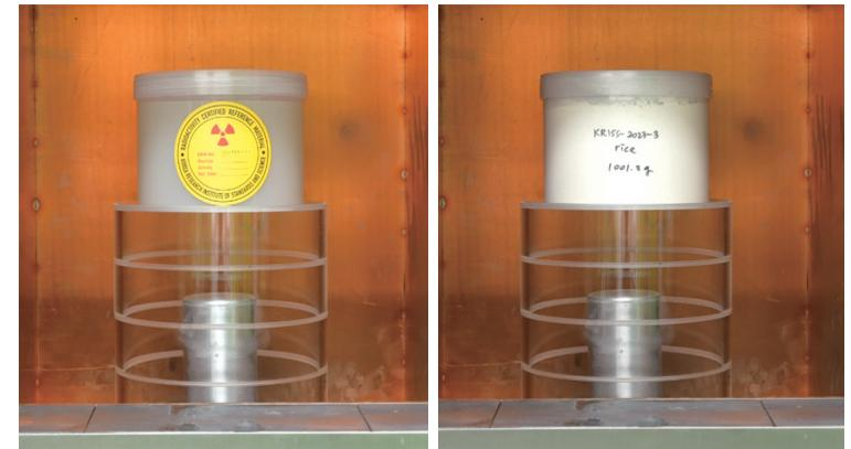
Figure 5. Calibration source and sample located at the same distance from the detector
