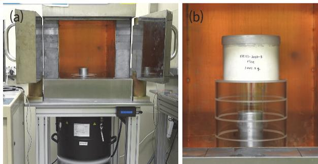
Figure 1. (a) A shield installed with the detector, and (b) increased distance between the detector and the sample
