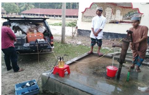
Measurement of Physical and Chemical Parameters of Groundwater, Bangladesh
